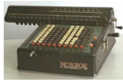
An early desktop "Monroe" calculator with a keyboard based number input which developed out of the typewriter technology
