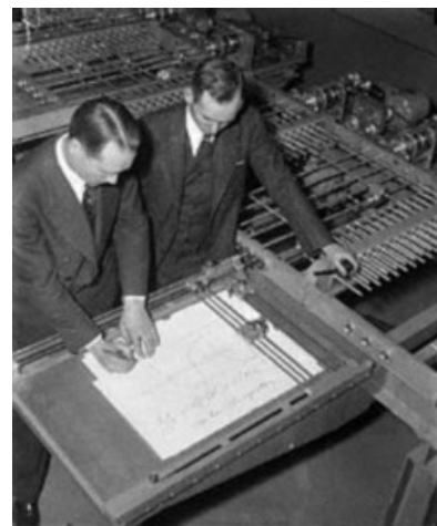
Vannevar Bush and his Differential Analyser - a analog mechanical computer that operated via mechanical line tracing by hand for input and automated graph drawing for output in 1923 [corbis image collection]
