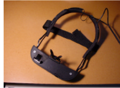
Commercial gaze tracker by ion - developed mainly to allow physically handicapped people to access the computer interface.
